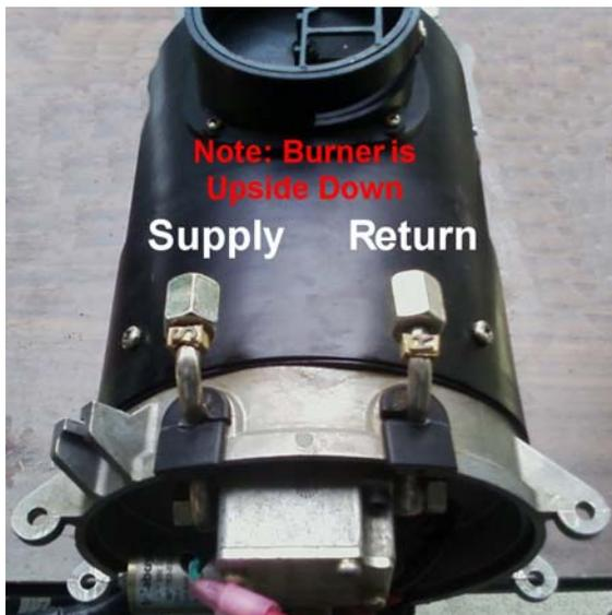
Use 12 mm open-end wrench on hose side and 14mm wrench on nut shown in photo left. The fuel hoses have been removed in this photo. Normally there will only be a couple of tablespoons of diesel fuel that will leak out when you remove the hoses. Have a towel handy. If fuel continues to drip, then either tie the hoses upright, or clamp them off with fuel pinch off pliers.
